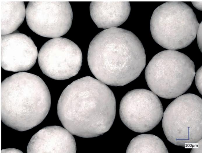
**Fig. 3** Poraver X features a closed-pore surface
