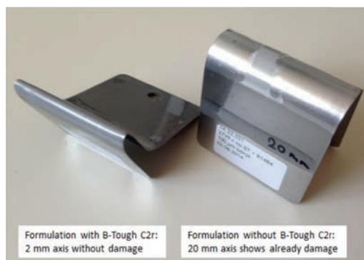
**Fig. 7 Flexibility and impact resistance results in formulations tested**
