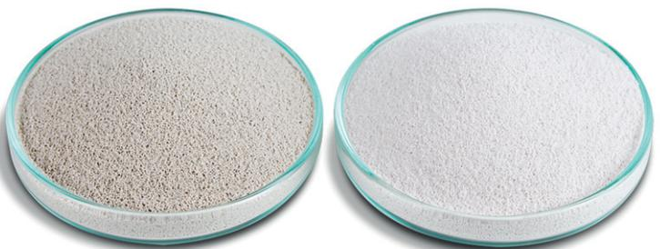
**Fig. 6** Colour comparison of Poraver (on left) and Poraver X granules
